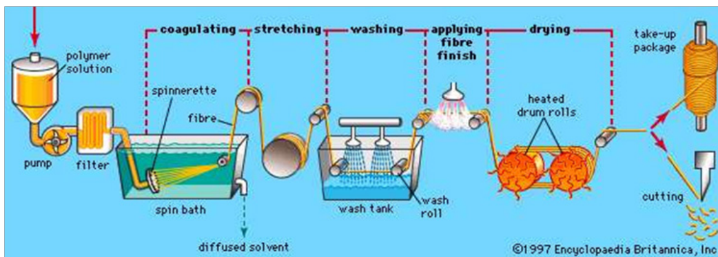
Figure : Stages in the wet spinning of polymeric fibres.
