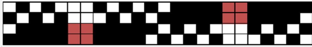
Figure: Bedford cord weave, 10 threads cord with 2 waded ends
